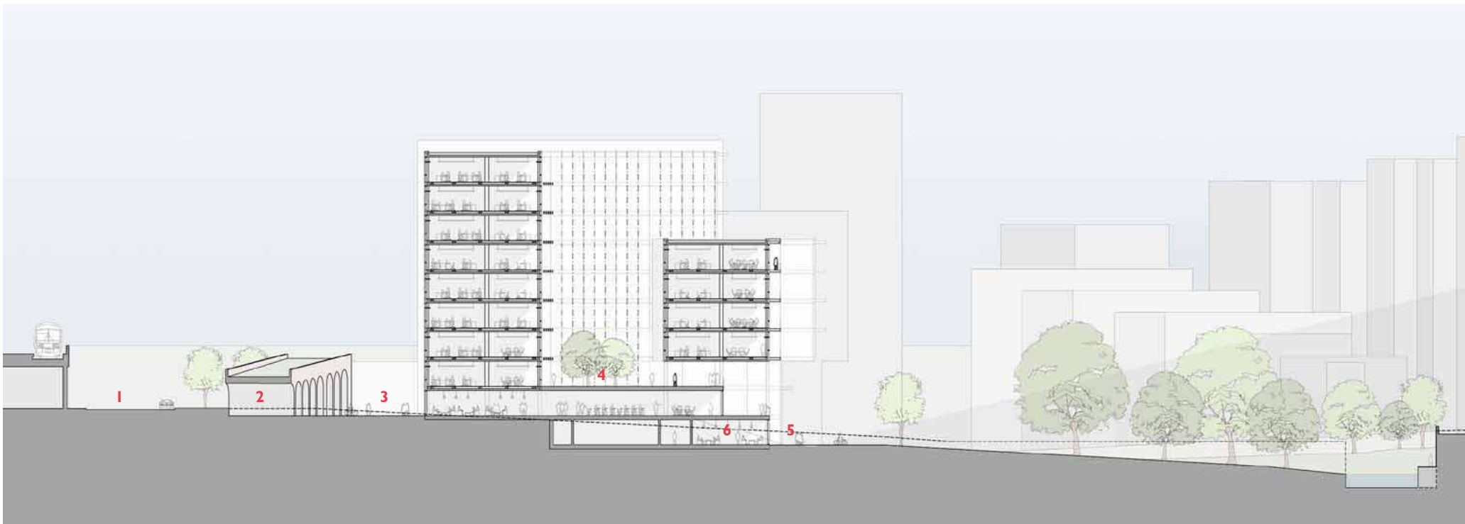
Section looking east - with sun angles and proposed height constraints for the Southern Development Zone to protect the quality of the park
