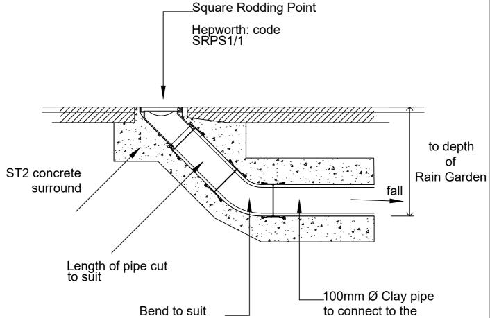
Hepworth clay drainage or similar approved components Pipe diameter to match land drain
