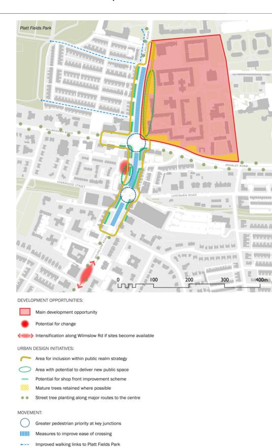
Figure 1: Fallowfield Action Plan key diagram
