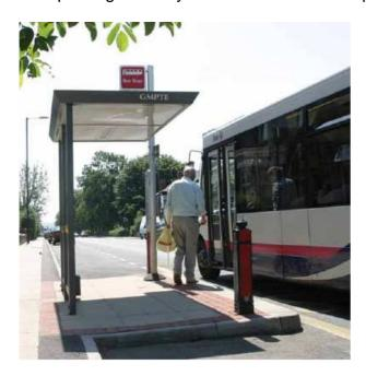
Bus boarders within indented bays greatly ease passenger access and bays provided on approaches to signals (as per example in Chorlton below) remove parked vehicles from the traffic stream and improve the capacity of signals for all users.
